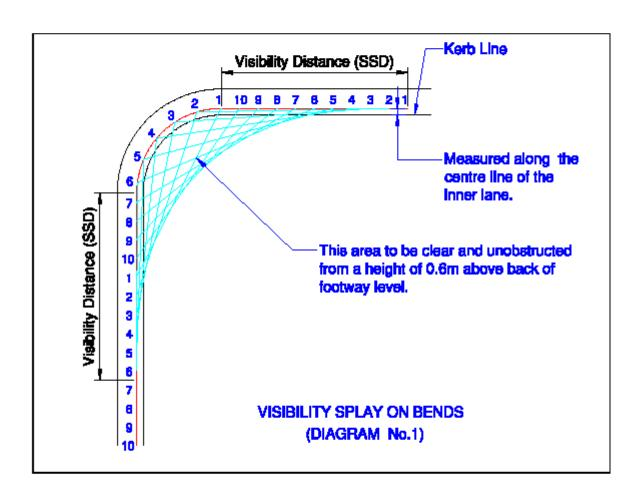
Parking bays should not be located within forward visibility lines and in visibility splays. The impact of street furniture on visibility should be assessed as part of the Road Safety Audits.
