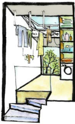
Fig. 47: Skylight over a laundry landing
