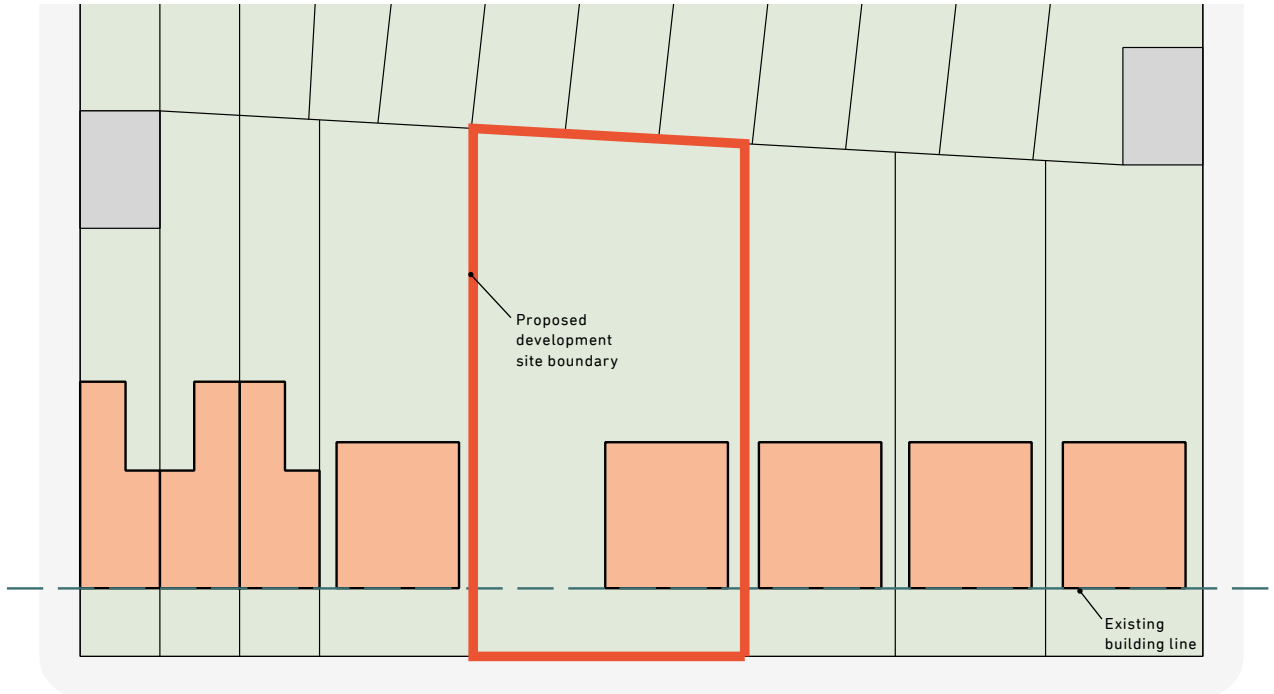
Fig. 99: Excessive gaps between existing houses provide an ideal opportunity for new homes whilst also enabling the streetscape to be repaired. These often occur on plots of land which are partially occupied by an existing property.
