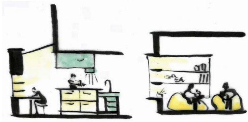
Fig. 52: High ceiling and large fanlight, good daylight to worktop and desks, well-lit living areas
