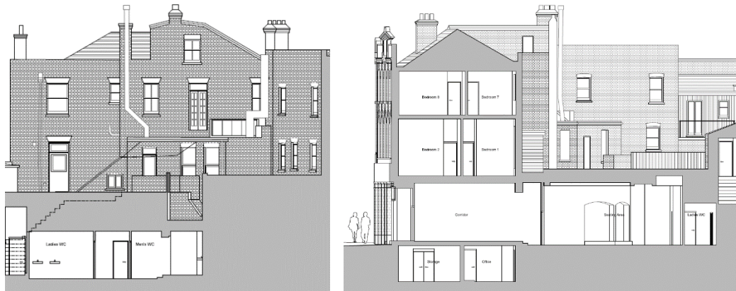
Figure 4.2 – Proposed rear elevation, with an improved flue arrangement, and sympathetic window alterations
