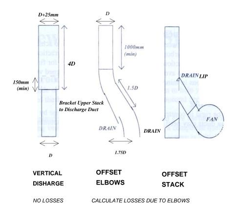
The rain penetration characteristics of these caps are superior to a deflecting cap located 0.75D from the top of the stack. The length of upper stack is related to rain protection. Excessive additional distance may cause "Blow-out" of effluent at the gap between upper and lower sections.
