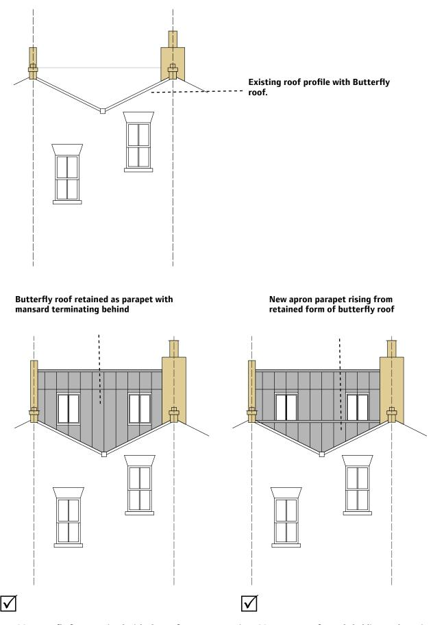
Fig 5.38:Butterfly form retained with slope of mansard running down to meet the existing eaves
