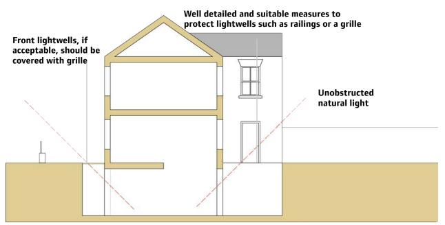
Fig 4.27: Section showing good practice and no impact on street
