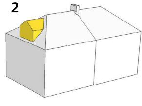
Fig 5.22: Properties 1 & 2 are acceptable outside conservation areas as they are significantly set in from all directions, are subordinate to the roof and match the existing roof profile
