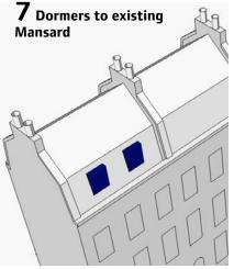
Fig 5.2: Types of roof extensions
