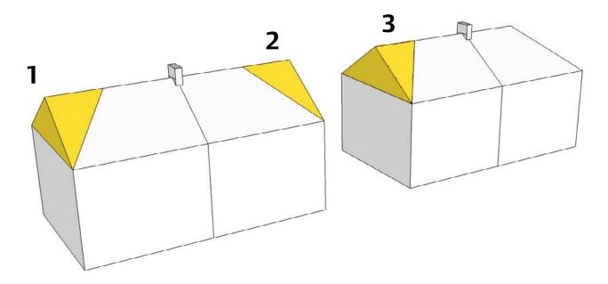
Fig 5.26: Properties 1 and 2 are acceptable outside of conservation areas as they maintain the symmetry of the semi-detached dwelling. Property 3 is acceptable outside of conservation areas as long as the sense of openess - if existing - is retained.
