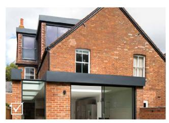
Fig 5.28: Acceptable due to sympathetic materials and they are both set in from the original roofline
