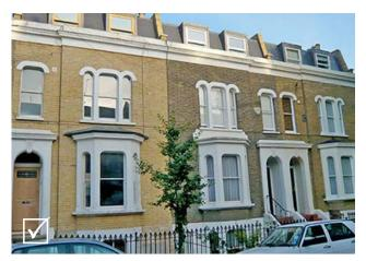
Fig 5.34: Acceptable example of mansard roof extension from the front behind existing parapet. All extensions are similar dimensions and look uniform
