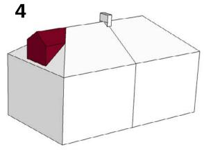
Fig 5.23: Property 3 is unacceptable as it does not complement the existing roof profile. Property 4 is unacceptable as it is not set down from the ridge line
