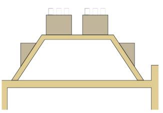
Fig 5.32: This is a modern variation of the traditional mansard roof form
