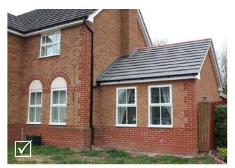
Fig 4.13: Sympathetic single storey side extension that steps back from original frontage.
