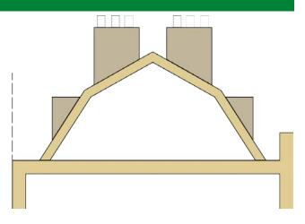
Fig 5.31: A double pitch mansard roof should have four slopes, the lower face should be steeply pitched and the upper slope should have a more shallow pitch. We would expect this traditional style Mansard within Conservation Areas where appropriate
