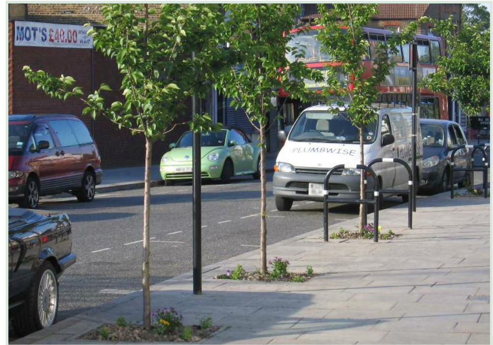
A single wider footway build-out can be a cheaper option.
