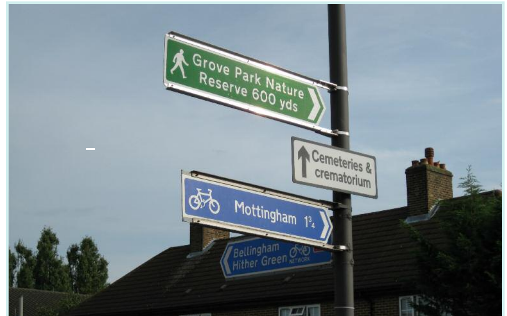
Cycle signs can sometimes be placed on street furniture to avoid erecting a separate post.
