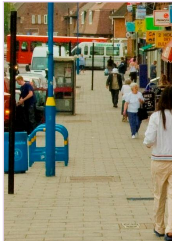
One way to increase the 'clear footway' is to cluster street furniture
