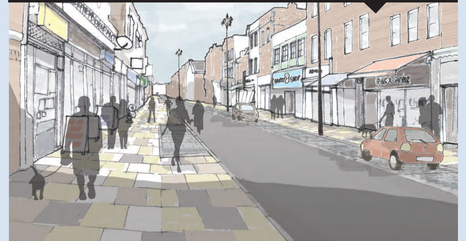
Example of introducing street furniture by reducing carriageway width Example of increasing footpath width to benefit pedestrian environment
