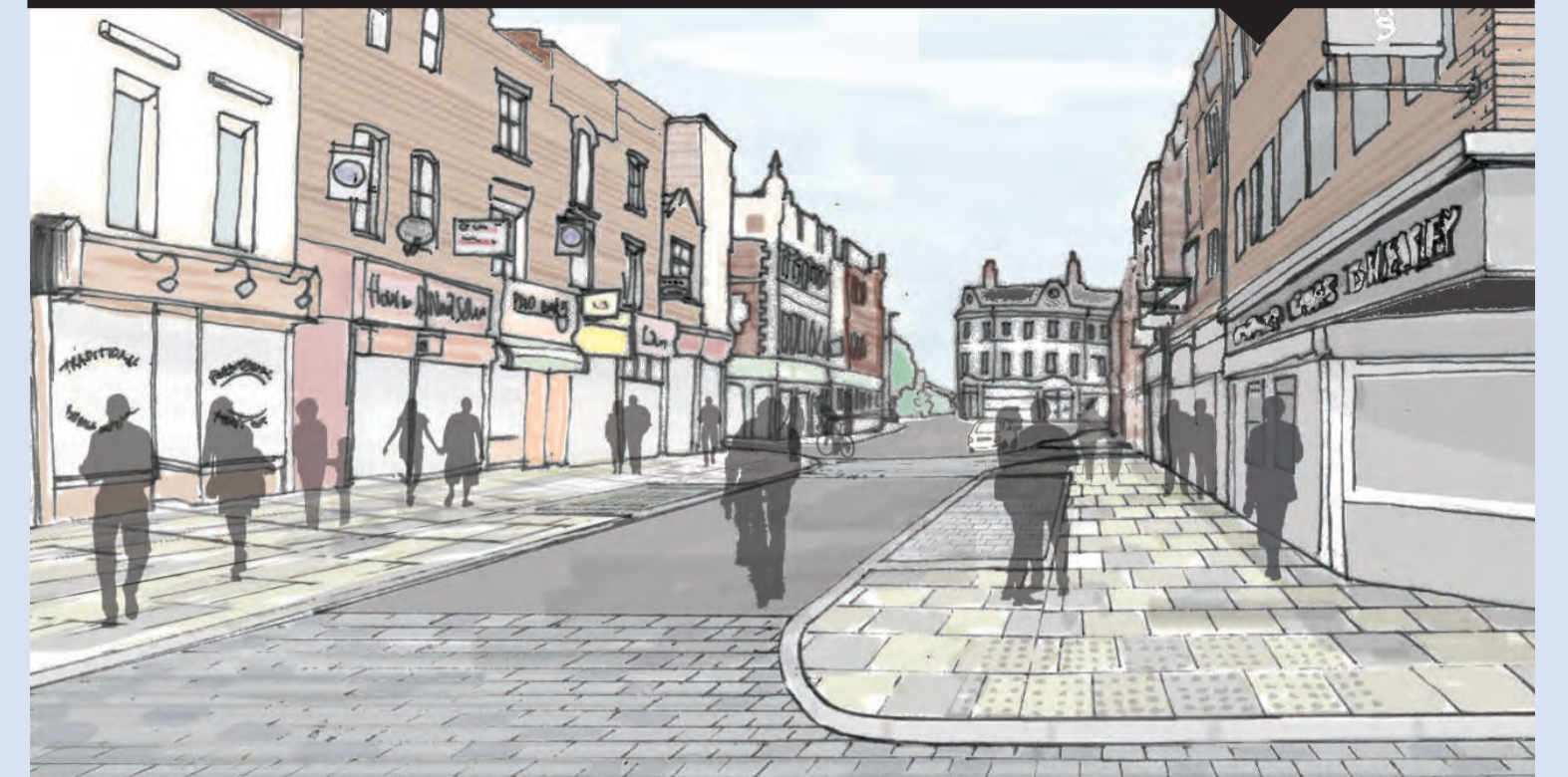
Example of parking and loading bays designed to be part of the footpath
