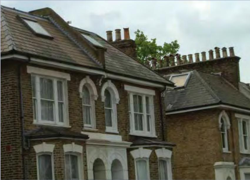
Intrusive rooflights of a modern design fitted proud of the roofslope
