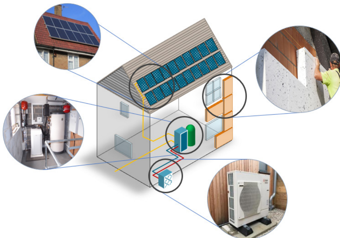
Figure 2.1: Whole system retrofit example: air source heat pump, solar PV and fabric retrofit
