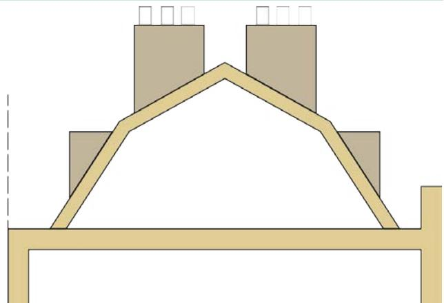
**Fig 5.31: A double pitch mansard roof should have four slopes, the lower face should be steeply pitched and the upper slope should have a more shallow pitch. We would expect this traditional style Mansard within Conservation Areas where appropriate**
