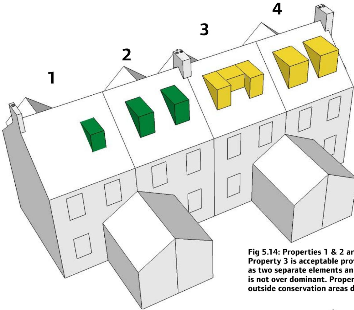
**Fig 5.14: Properties 1 & 2 are acceptable in all areas. Property 3 is acceptable providing the dormers read as two separate elements and the central connector is not over dominant. Property 4 is only acceptable outside conservation areas due to their size and bulk**
