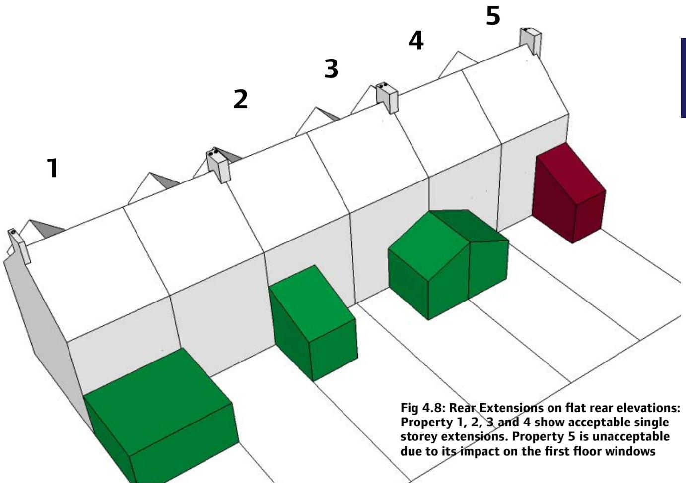
**Fig 4.8: Rear Extensions on flat rear elevations: Property 1, 2, 3 and 4 show acceptable single storey extensions. Property 5 is unacceptable due to its impact on the first floor windows**
