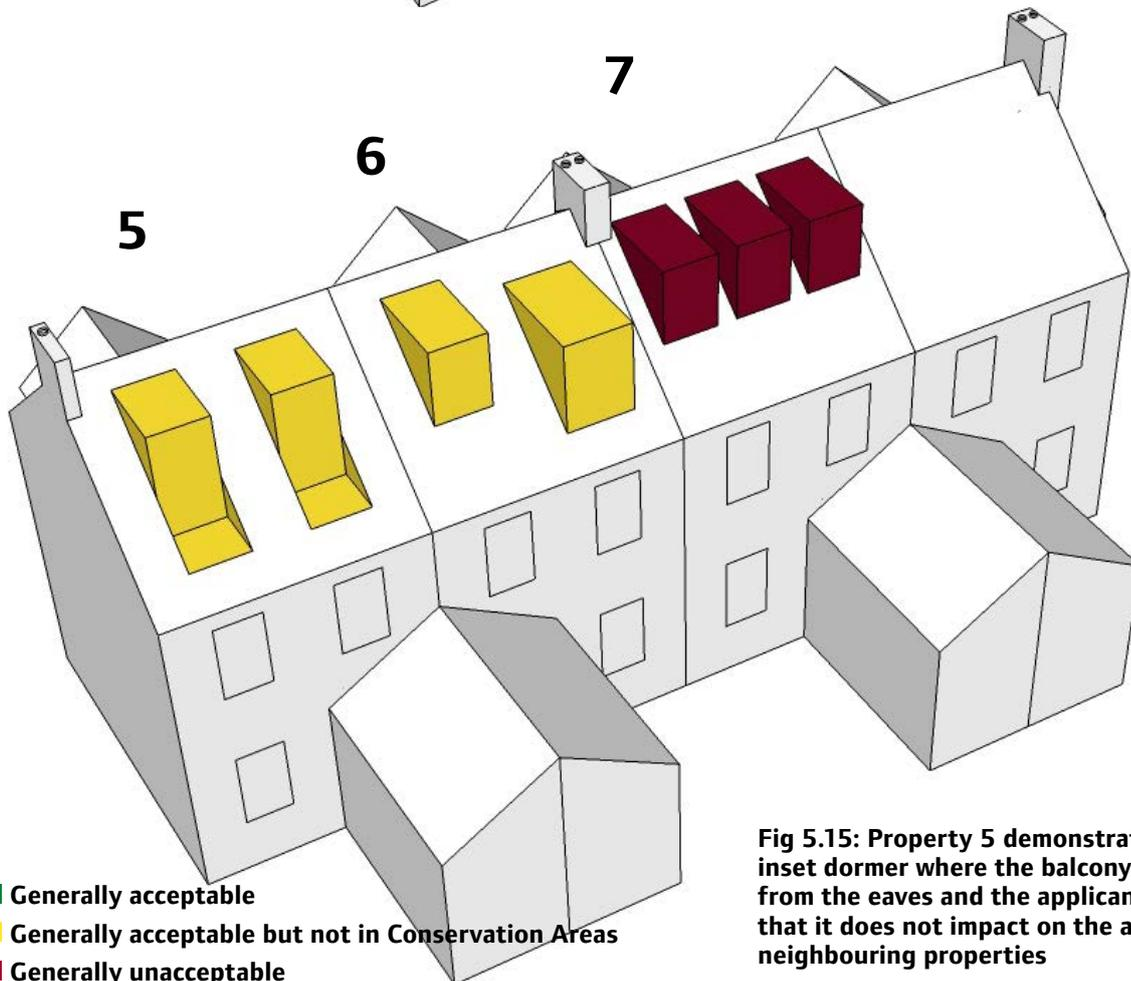
**Fig 5.15: Property 5 demonstrates an acceptable inset dormer where the balcony is inset significantly from the eaves and the applicant has demonstrated that it does not impact on the amenity of neighbouring properties**
