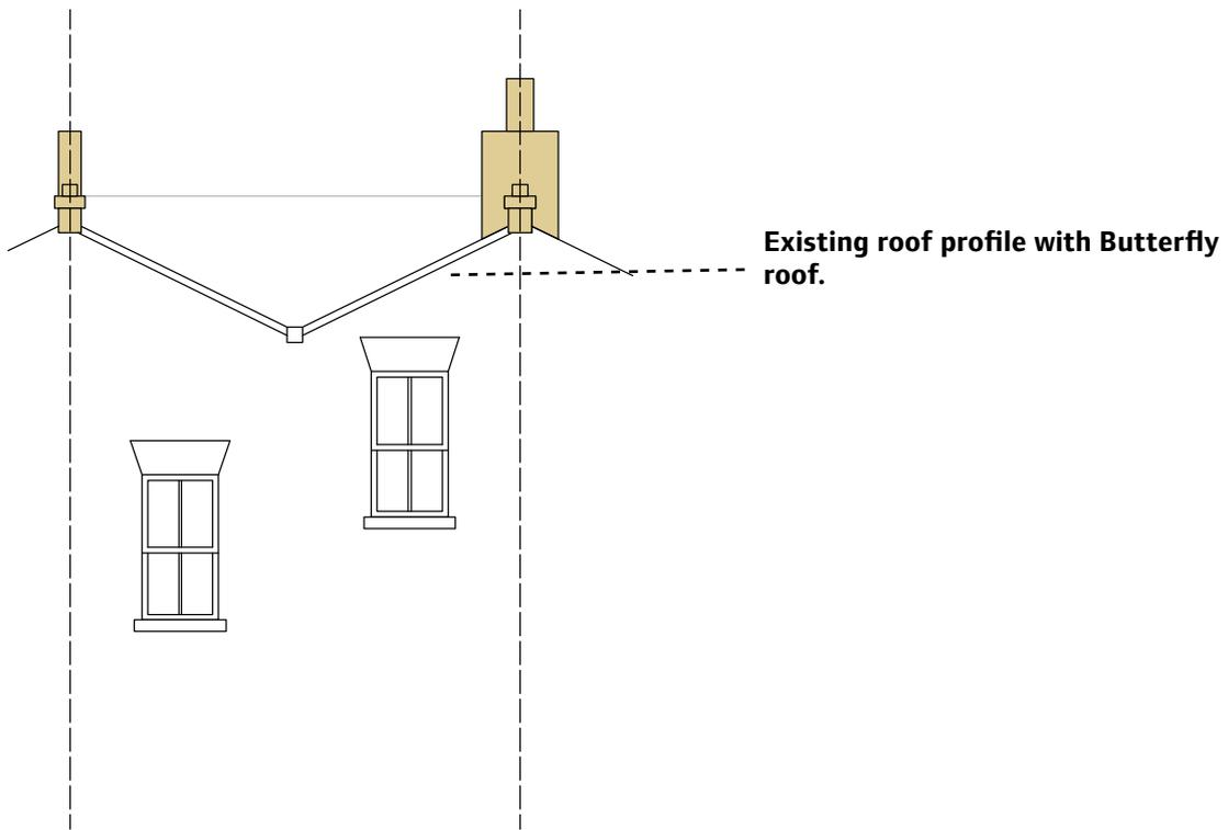
Butterfly roof retained as parapet with mansard terminating behind
