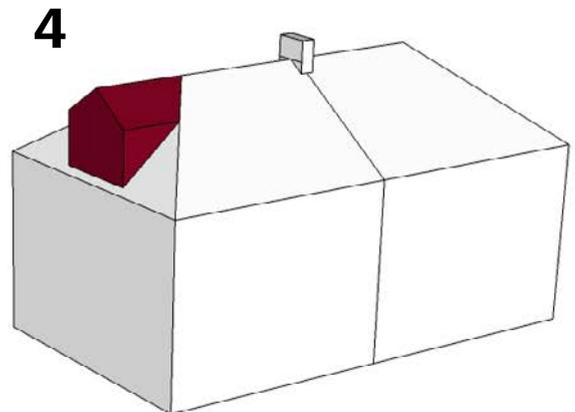
Fig 5.23: Property 3 is unacceptable as it does not complement the existing roof profile. Property 4 is unacceptable as it is not set down from the ridge line
