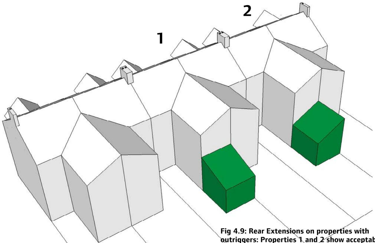
**Fig 4.9: Rear Extensions on properties with outriggers: Properties 1 and 2 show acceptable extensions as they do not substantially extend on the garden and are not overbearing on neighbouring properties**
