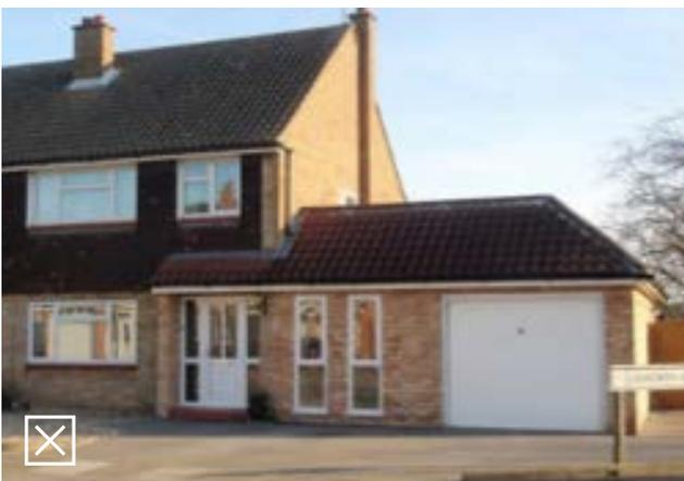
**Fig 4.12: Unacceptable because the side extension is more than half the width of original house and is not set back from original frontage**
