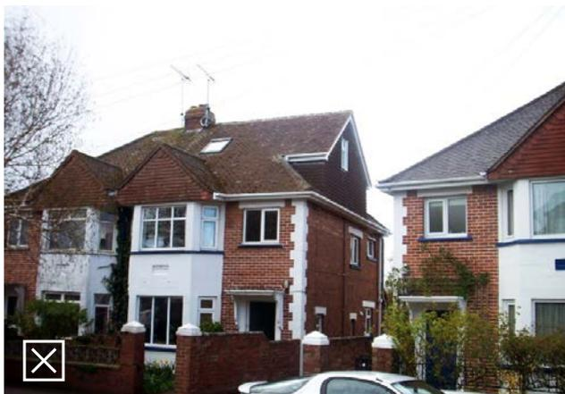
**Fig 5.20: Unacceptable as the side dormer alters the symmetry of the pair and harms the original design integrity of the existing building**
