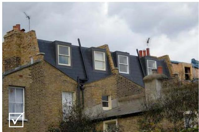
**Fig 5.37: Acceptable - Butterfly form retained with slope of mansard running down to meet the existing eaves (please note that proposals should not include drainpipes)**
