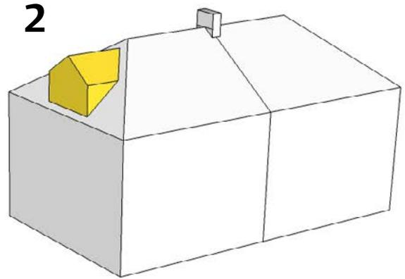
Fig 5.22: Properties 1 & 2 are acceptable outside conservation areas as they are significantly set in from all directions, are subordinate to the roof and match the existing roof profile
