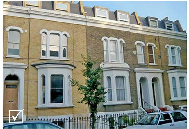
**Fig 5.34: Acceptable example of mansard roof extension from the front behind existing parapet. All extensions are similar dimensions and look uniform**
