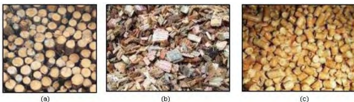
Figure B-3 Wood fuel types: (a) Logs; (b) Chips; (c) Pellets
