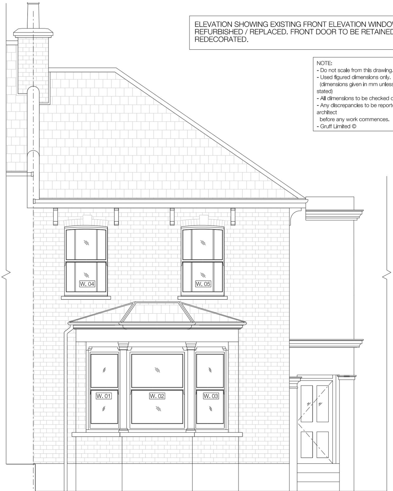
ELEVATION SHOWING EXISTING FRONT ELEVATION WINDOWS TO BE REFURBISHED / REPLACED. FRONT DOOR TO BE RETAINED BUT REDECORATED.
