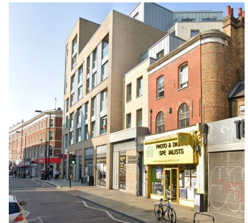
Principle: Along retail parades, encourage taller ground floor ceiling heights to be adaptable to retail Precedent: New developments along Kingsland Road, LB Hackney
