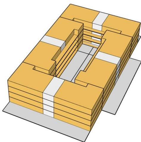
**Figure 4.14 SketchUp model showing a perimeter block using four linear blocks**
